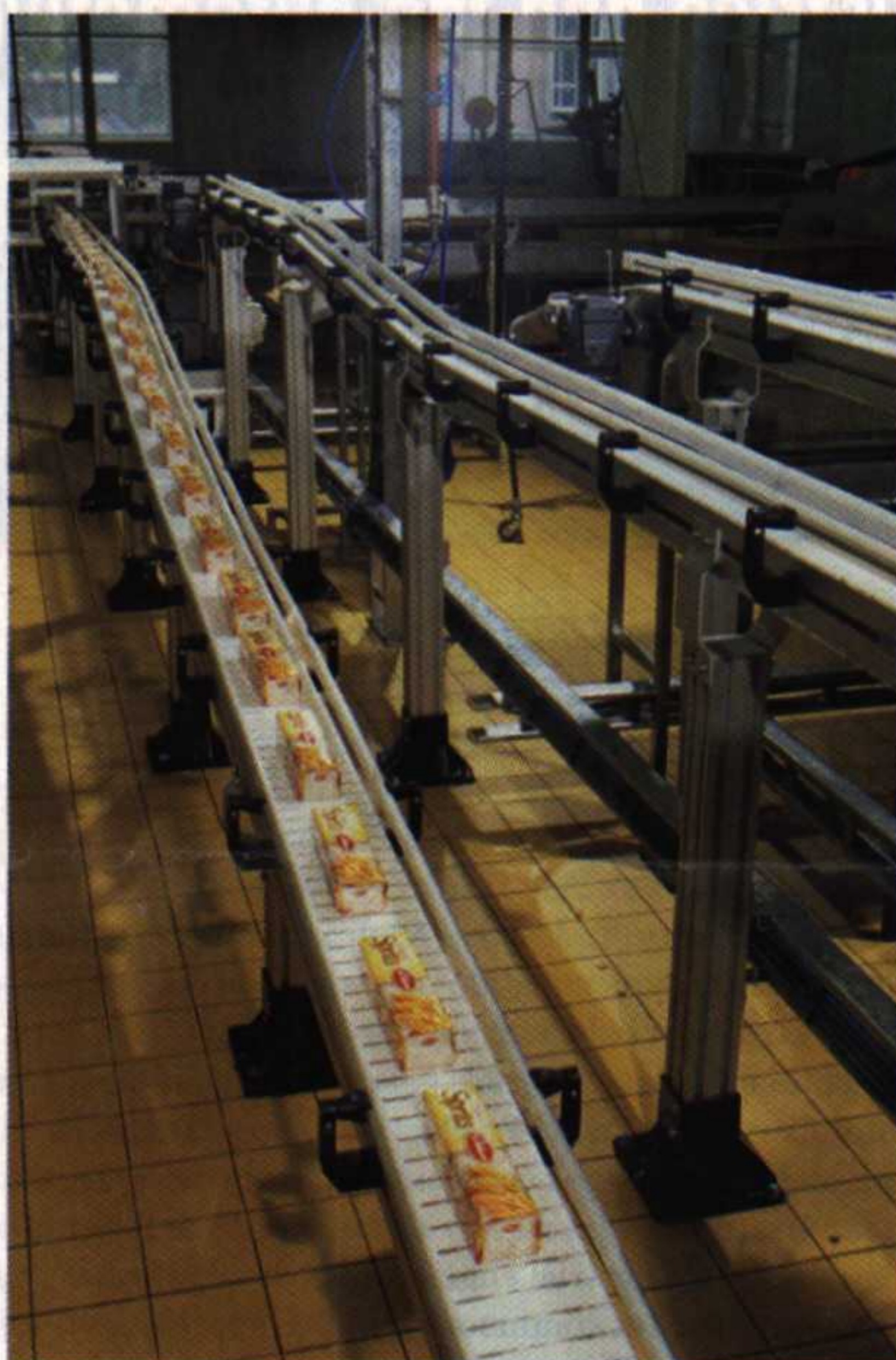
■ Conveyors for buffering and for non-value-added conveying of finished goods such as biscuits are appropriate uses of technology in a lean environment because they free people to perform high-value tasks. Source: Bosch Rexroth Corp.
